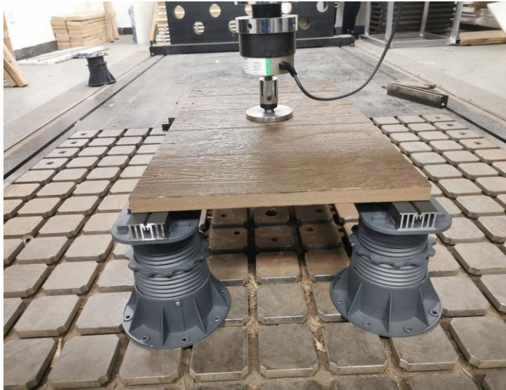
Fig.1 Test set with 25mm beams
