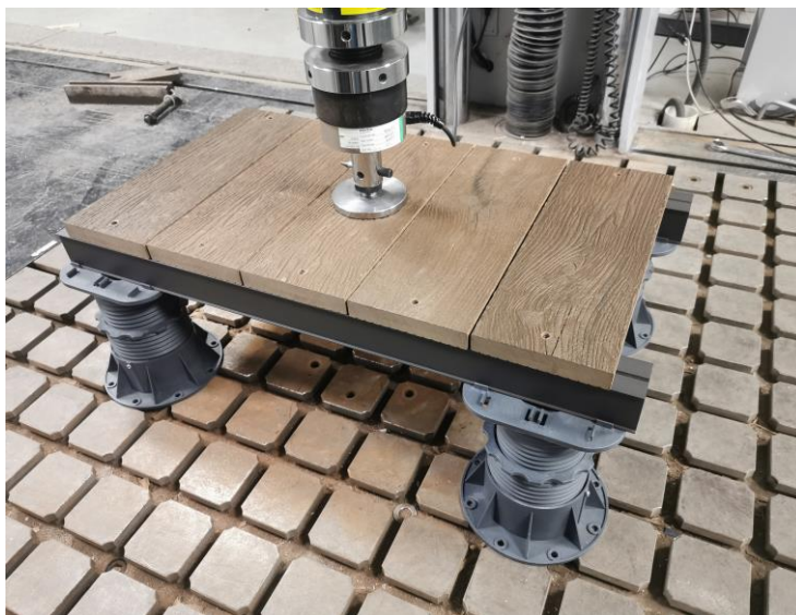
Fig.2 Test set with 50mm beams
