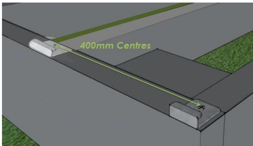
Boards should be fixed with clips on each bearer/joist. Clips should be fixed no further than 400mm apart down each side of the board. Clips should be fixed no less than 10mm in from the end of the boards (this will stop the boards falling off the clip, on contraction). Installation of hollow boards **MUST** use the fixing kits provided by Saige Longlife Decking.
