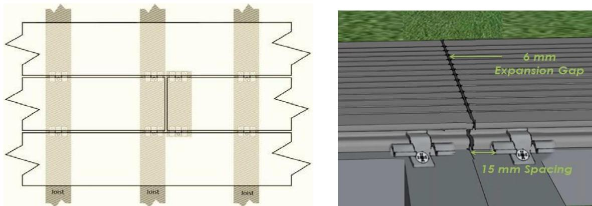
For the first board, install to the baton as detailed above. For the second board, attach a second board on a second baton/joist – as above diagram.
